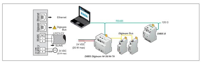
(\*) If the 24 VDC power supply is not provided by Socomec, a 1 A / 24 VDC fuse must be used. For North America, the use of recognized fuses is mandatory.
