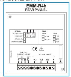
REMARKS: It's a must to respect the phase sequence. The connections between current and voltage phase inputs must not be inverted (for example, CT placed on phase L1 must correspond to the I1 input). So as it is not correct to invert S1 and S2 terminals, since power factors and powers might not be reliable.
