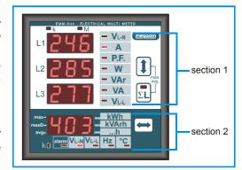
Press **A** button to see on **F** display the three phase value (the average of the single phase of voltage, current, power factor and the sum of single phase for the power) of the parameter selected: the led inside the **A** key is on.
