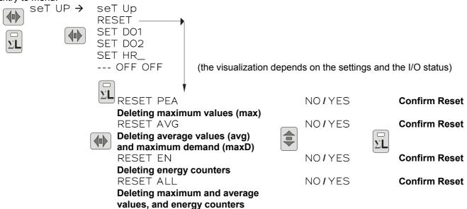
To enable the chosen type, press the **B** key to change the indication on display **G** from NO to yes. Confirm enabling cancellation, by pressing the **A** key. The indication on display **G** change from yes to --- .
